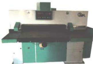
Semi Automatic Paper Cutting Machine with Electromagnetic Clutch
